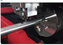
Equipped with a chuck index, it's possible to process not only flat plates but also tubes.
