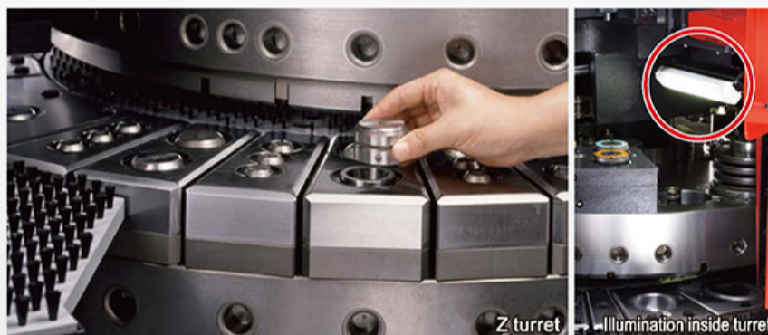
Illumination inside turret A work light illuminates the inside of the turret during a tool change.
