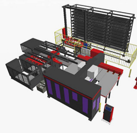
EM-ZR + takeout loader + material and part warehouse
